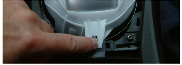
3. Pry shift cable ball end off of side-to side lever and let cable-end rest at bottom. Pry shift cable ball end off of shifter bottom, let cable end rest at bottom.
