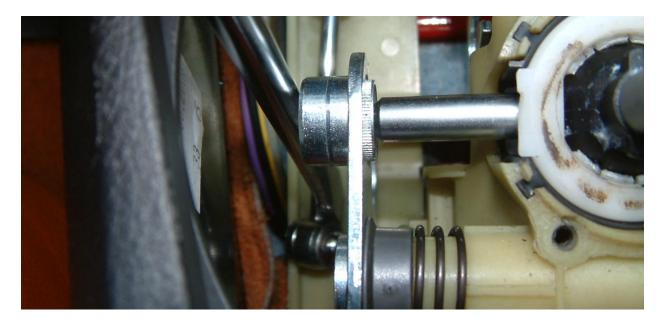
4. "Remove three Torx screws from top of Shifter Base (white plastic base) to remove Round Cover (Black Plastic), then remove Upper Socket Spacer (white plastic, with slots) and set aside.
