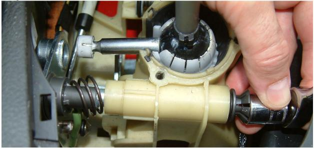
7. Modify shifter base to allow new shifter cable position with sharp chisel or grinder. Remove rib as shown.
