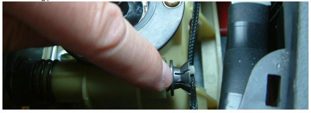
Using small socket to flare out the tabs on the clip
