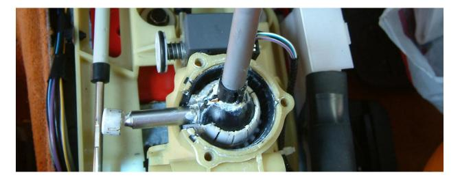
6. Remove spring clip for side-to-side lever by flexing tabs on clip to allow rod to slide to left. *Tip: An easy way to release clip is to push all tabs with a small socket, while pulling lever to the left.(If Clip tabs break off, there is a new Clip in the kit).* See following pictures.
