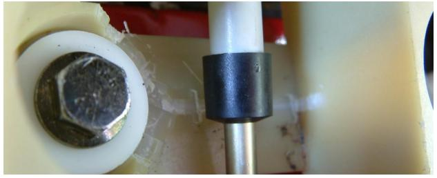
8. To remove shift stick, push side-to-side rod to left, and pull shifter upwards to release from socket.
