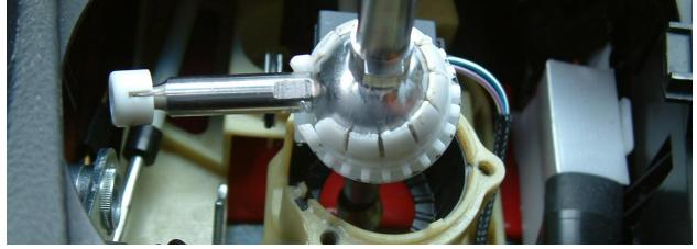
11. Fit SNABB stick into recess, then re-fit forward-backward cable end to stick, you will hear a sharp click or snap when it is on correctly.
