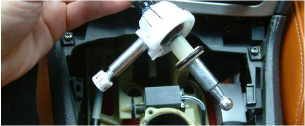
9. Pry or pull white plastic ball bushing from shifter. Remove small white plastic bushing from side rod and remove O-ring from shifter bottom.
