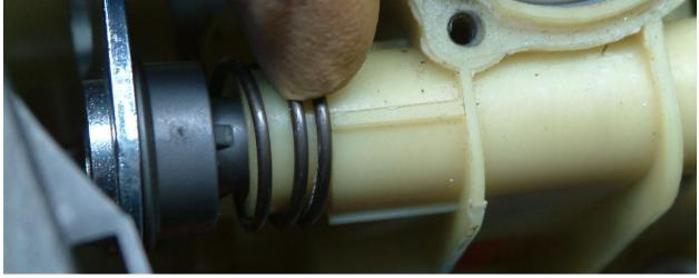
\*Note\* see above photo for correct orientation of grey plastic bushing, rib must be straight up.
