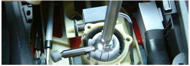
12. Refit top retaining Upper Socket Spacer and Top (round) Cover, and refit 3 Torx screws. Do Not Over-tighten
