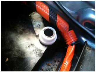
6. Place the assembly over the spindles and new bushings then place the set of Delrin washers on top of the holes. Place the metal inserts in through the washer.
