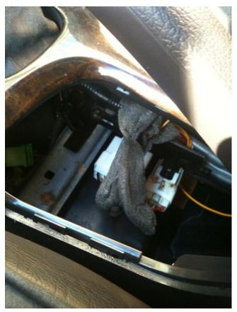
6. The console should be ready to remove now. Make sure that nothing else is attached, then pull up on the from the back first and slide backwards to release. Pull the console up and out while positioning the shift boot so that it will slide down through the hole in the console.
