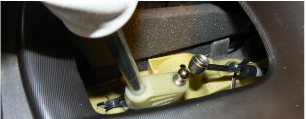
2. Place both parts of the adapter onto the shaft just under the boot where it can be easily reached. (Make sure that the alignment of the small piece is correct as it is not perfectly symmetrical: You want the back edge of the two pieces to be flush when mounted on the shaft so that the bolts align correctly and do not get cross threaded) Thread the (4) bolts by hand until they are mostly in but still loose enough that you can slide the adapter down on the shaft.
