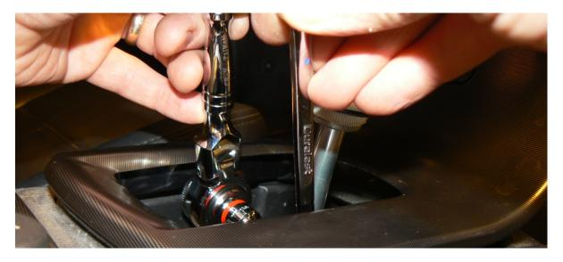
6. Push cable end onto the ball.
