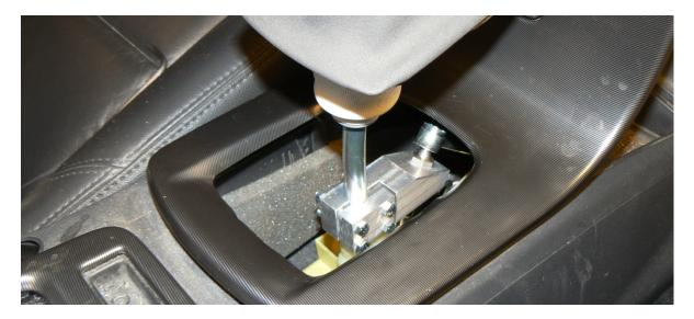
\*\*Please note that raising or lowering the adapter on the shaft will slightly alter whether the shift lever is perfectly straight up and down. For this reason there is a small amount of adjustment available on the ball location. For example: If you find that the shifter is slightly forward you can remove the ball with ½ drive socket and wrench and move the ball reward to straighten the shift lever and vice versa. There is approximately 1 inch (shift knob travel) of total adjustment available.
