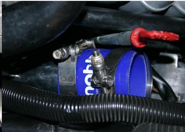
Install the 2.25" straight coupler to the top of the lower IC inlet pipe with a supplied 2.56" Tbolt, tighten all the way. (Above right)
