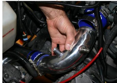
Position the 90 degree throttle body pipe into the Throttle body coupler and into the 2.5" coupler from the lower FMIC outlet pipe. Position it so that it is snug up against the lower coolant pipe then tighten all the clamps on the outlet side. (Remember to tighten the IC outlet clamps that you didn't tighten earlier) (below left..next page)
