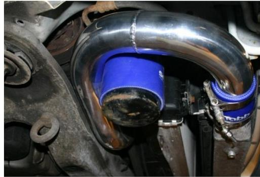
**Installing Bottom Intercooler outlet pipe:**
