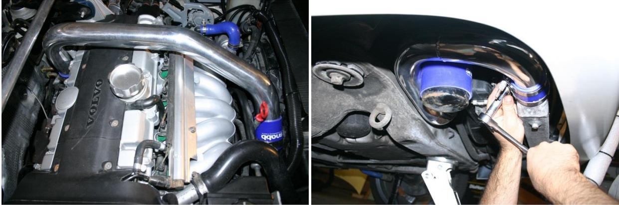
Install upper IC inlet pipe into the two silicone couplers along with 2.56" t-bolts on each side. Position the Tbolts as shown and tighten down all the way if everything is aligned correctly. If not, reposition as needed then, tighten clamps. Now go back and finish tightening the bottom IC inlet clamps that you left loose. (see above)
