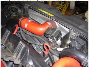
Use 1/8<sup>th</sup> drive rachet with 7mm socket to remove clamps
