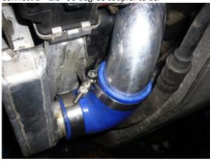
Install TTP & connect to LCP with 2.75">2.5" coupler
