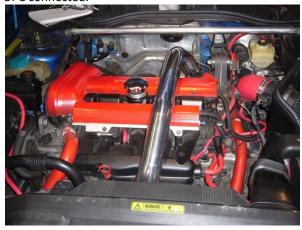
Once you have finished installing the RIP kit, reinstall the radiator trim piece, airbox inlet and then reconnect the negative terminal of the battery.
