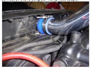
Connect UCP to Turbo using 2"<2.5" coupler
