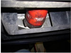
Remove large VAC line from nipple on Charge piping
