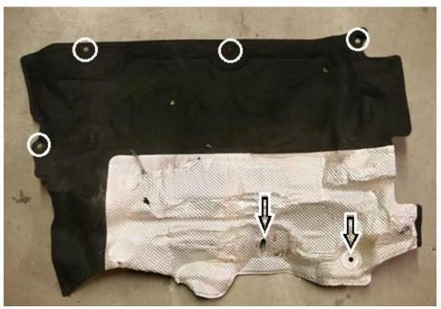
3. Remove (5) 8mm bolts on the metal panel: 2 on passenger side and 3 on drivers' side. Before fully removing the panel the metal tabs (if your car has them) will be located on the bottom of the plate need to be released. Slightly pull forward and up on the passenger's, then the driver's side of the metal panel. The protective metal panel can now be removed from the engine bay.
