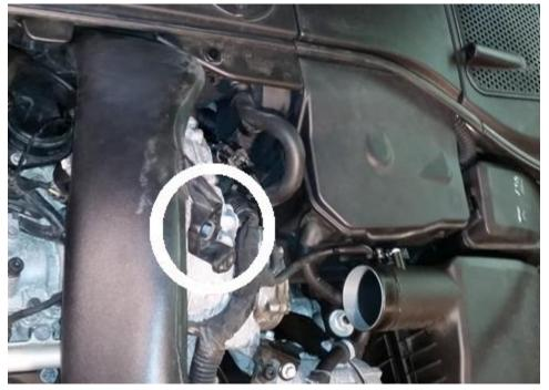
7. Located behind the CVC, remove the M6 Bolt holding the upper intake mounting bracket.
