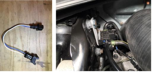
3. Install the 1 ½" x ½" straight bracket to secure the electrical connector that used to be attached to the OEM intake pipe. Use the 2<sup>nd</sup> M6x20 bolt and M6 lock washer to attach the bracket as shown to the threaded hole on the timing cover and then push the barbed tab on the connector into the upper hole until it locks in place.
