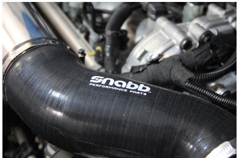
6. Positioning the pipe: while the WD40 is still wet position the aluminum intake so that the bracket is lined up with the bolt hole that is directly below it on the engine cam cover. Once the slot on the intake pipe is lined up correctly with the bolt hole (so that the bolt will be centered in the slot and positioned toward the back of the slot) use the M6x 20 Bolt and black nylon washer to tighten the pipe to the cam cover. Now you can position the hoses so that they are fully
