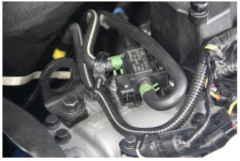
3. Disconnect and remove the 5mm hose that runs from the TCV to the upper section of the intake pipe (near the joint for upper and lower intake pipes).
