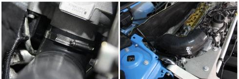
2. Place the TCV bracket over the large M12 bolt that holds the upper torque mount to the unibody mounting point. Install the included M12 jam nut nut to tighten down the bracket to the bolt. Plug the TCV wiring harness extension onto the OEM harness and the TCV. Install TCV onto the bracket with the electrical connector facing the firewall. Replace the TCV vent hose (to the intake pipe) with the longer 17" long section, run the hose and the wiring harness extension
