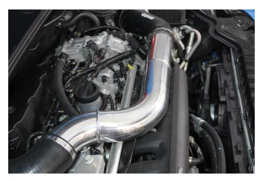
5. Take the 3" S shaped silicone hose for the MAF, lubricate the inside of it with WD40. Place a #48 clamp on either end of the hose and then install the hose onto the MAF and the other intake pipe.
