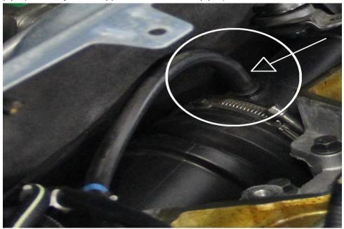
4. Remove the breather-hose clamp from the crankcase ventilation cover (CVC) and upper intake pipe then remove and discard the short 14mm hose that connects the breather box to the intake pipe.
