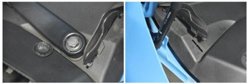
4. Using a pair of needle nose pliers and a small flat head screwdriver remove the six plastic clips that hold the plastic drainage cover.
