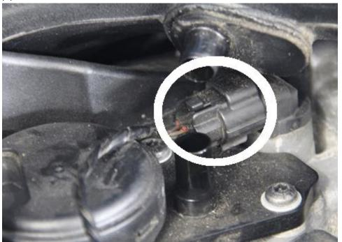
6. On the cam chain side of the motor, remove the M6 bolt that holds the upper intake pipe to the side of the engine block, and remove the electrical connector that is attached to the intake pipe
