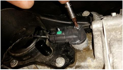
2. Using the T30 bit and a 10mm socket, remove the (12) M6 bolts holding the CVC to the engine.
