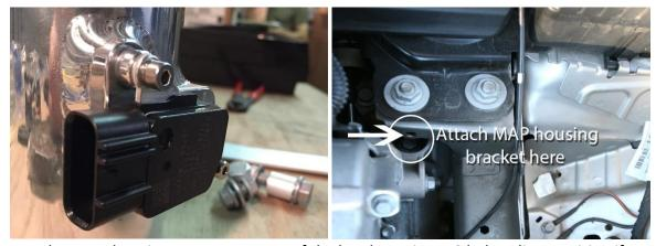
• Attach sensor housing onto upper part of the bracket using M8 bolt- adjust position if needed and don't forget to plug the sensor back in!
