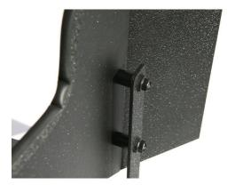
Once the airbox is in place, use the remaining L bracket hardware (Kit 1) to attach bracket to airbox: See pics Above.
