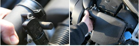
Remove the rubber and plastic foot from the lower frame rail bracket. REMOVE THE RUBBER GROMMET ON THE BACK OF THE AIRBOX AND SET ASIDE, you will need it in next step.
