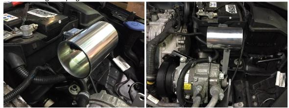
• Attach the airfilter to the sensor housing , then attach intake pipe to sensor housing and tighten down both clamps.
