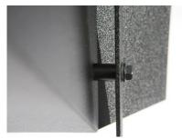
At this point the heatshield is installed and should be secured to the vehicle.
