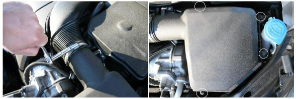
• Disconnect the electrical connector from the air mass sensor in the airbox lid, then remove the 2 (T15) screws from sensor to remove it from the lid. Put the air mass sensor aside for reinstallation into the new kit.
