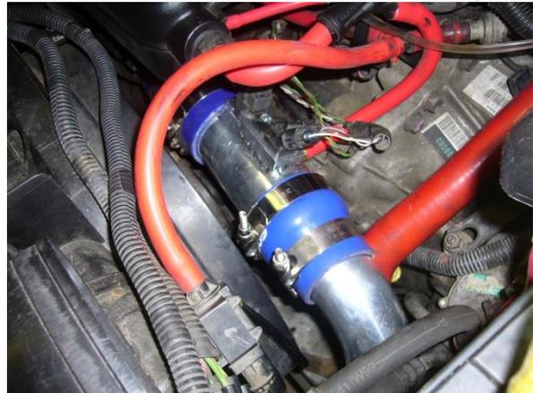
Connect UPC to IC using 2.5" hump hose coupler
