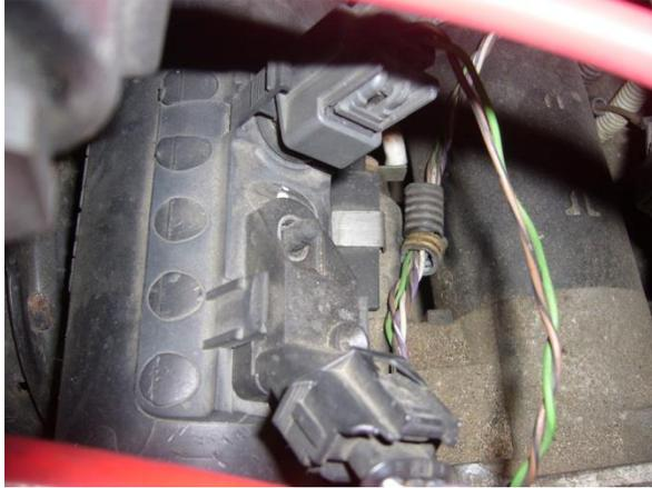
Install sensors into TTP: Secure MAP with M6x12 bolt
