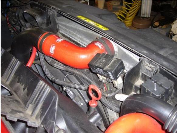
Removing lower (stock) IC connector
