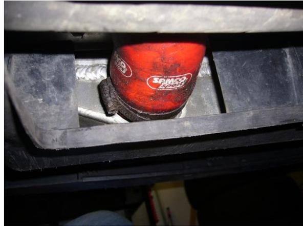
Use 1/8<sup>th</sup> drive ratchet with 7mm socket to remove clamps
