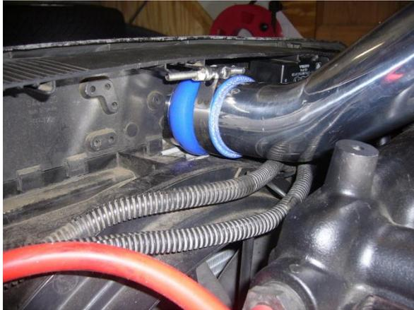
Connect UCP to Turbo using 2" < 2.5" coupler
