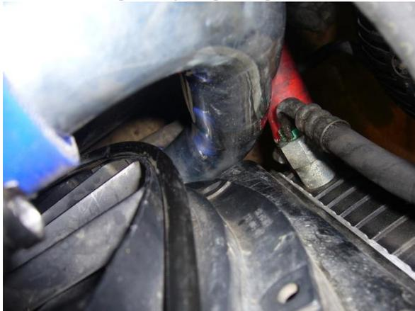
Install TTP & connect to LCP with 2.75" > 2.5" coupler
