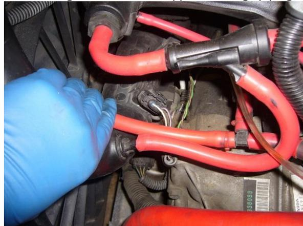
NOTE For the next step: Be careful when removing the IAT sensor (with 2 plastic side clips) from your factory cold side charge air pipe. You will need to gently loosen and remove the IAT sensor because you need the clips intact to reinstall it into your new Snabb RIP kit cold side piping. Note you may want to use a little soapy water to aid with the install of the sensors into the Snabb TTP.
