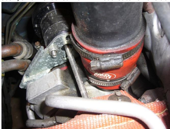
Use 1/8 th drive ratchet with 7mm socket to remove clamps
