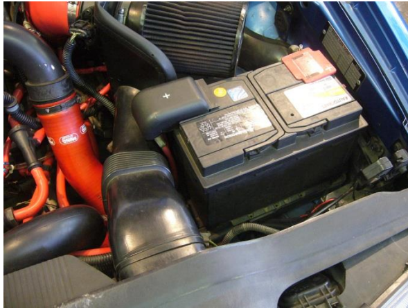
Pull up to remove trim piece for access to IC inlet
