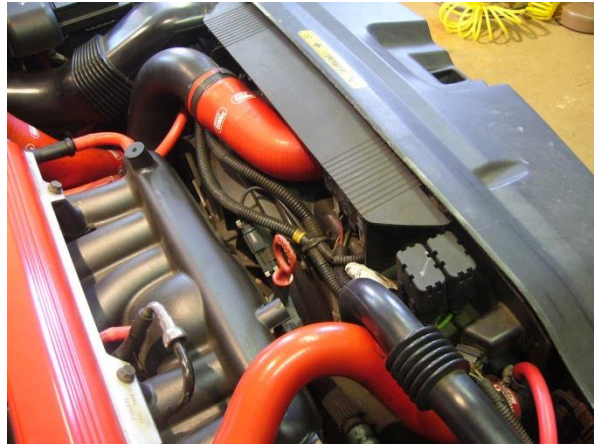
Removing lower (stock) IC connector
