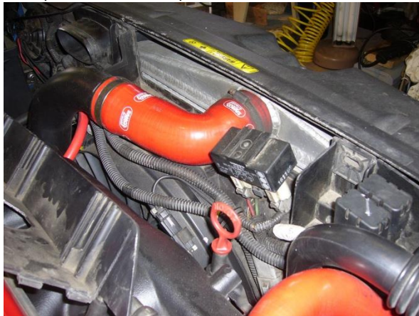
Use 1/8 th drive ratchet with 7mm socket to remove clamps
